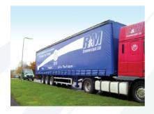
Side Curtains can be provided in a wide variety of colours made in a top quality 900g PVC. We can also supply insulated or mesh curtains.
